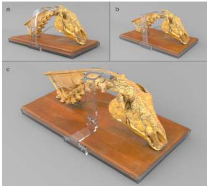
Fig. 6. 3D models of different supports considered during the computer design phase: a) support with one-piece curved arm; b) support with one-piece right-angled arm; c) support with adjustable arm
