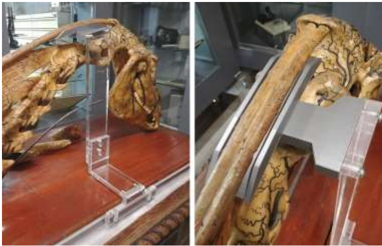
Fig. 8. Functional test with the upper part of the support printed in PLA
