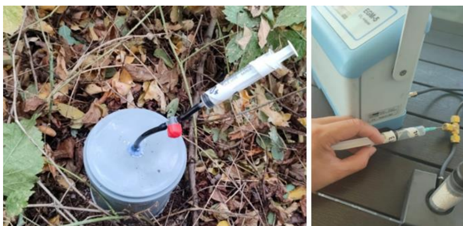
Fig. 4. Injection kit for carbon dioxide collecting and the analysis process
