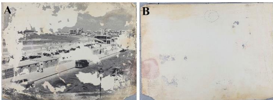
Fig. 2. Photograph C; The photograph from which B. amyloliquefacien was isolated, showing signs of deterioration: a) losses in gelatin binder, b) color stains in the back
