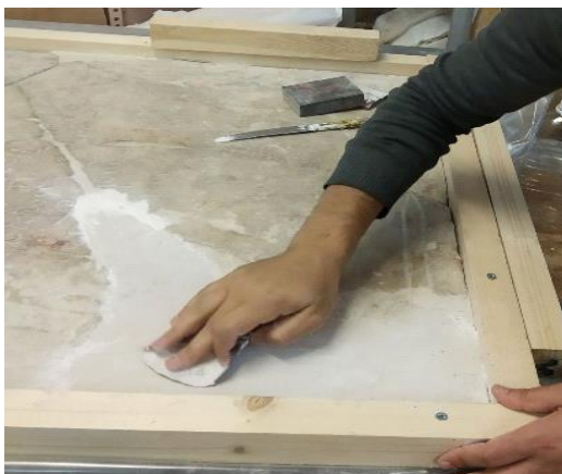
Fig. 7. Sanding the stone surface with sandpaper.
