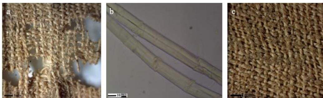
**Fig. 9.** Investigation of the textile: (a) Deterioration aspects of insect's attack. (b) Textile is identified as linen. (c) Textile quality  $16 \times 24$  threads per  $1\text{cm}^2$
