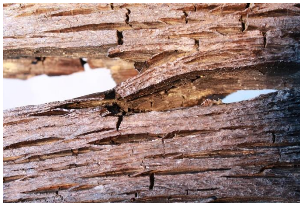
Fig. 5. Visible are numerous deformations as well as longitudinal and transverse cracks of the wood in the stern, formed during the storage of the boat in the outbuilding. Photo: M. Aniszewski
