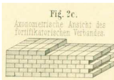
Fig. 7. The way of arranging bricks with the head facing the front of the wall. The so-called fortress binding of the wall ( Fortifikatorischer Verband ), Source of illustration: Constructions-Details der Kriegs-Baukunst, Band I , Wien 1878; Table No. 4 "Mauern, verschiedene Ziegel-Verbände".
