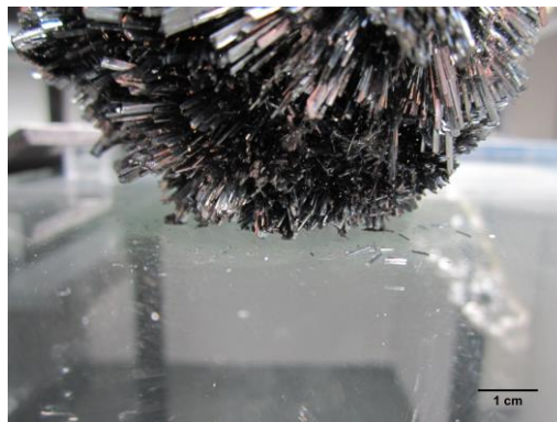
Fig. 10. Detail of Stibnite surface abrasion due to incorrect support/gravitational forces on the projecting structures inside a showcase-type-A. MUHNAC-ULisboa, Coleções de Mineralogia, n° inv: MNHN/UL.7358. Image taken on 28/08/2020
