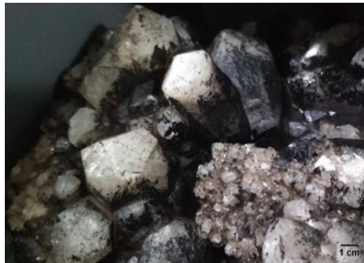
Fig. 12. An example of Calcite affected by smoke and black soot from the fire. MUHNAC-ULisboa, Colecções de Mineralogia, nº inv: MNHN/UL.1473. Image taken on 13/02/2020.
