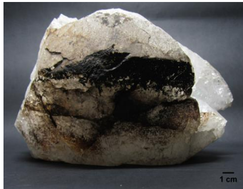
Fig. 11. An example of a fragmented Quartz affected by smoke and black soot and material loss from the fire. This specimen is no longer part of the collection; serves as an exemplification of the fire damage. Image taken on 13/02/2020.
