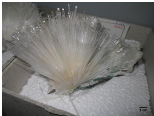
Fig. 9. A detail of Mesolite with Styrofoam® base and surface abrasion/material loss on the projecting structures. MUHNAC-ULisboa, Coleções de Mineralogia, n° inv: MNHN/UL.8847. Image taken on 15/07/2020
