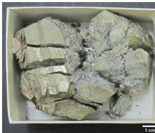
Fig. 6. Pyrite decay. MUHNAC-ULisboa, Coleções de Mineralogia, n° inv: MNHN/UL.7280. Image taken on 15/02/2019. This mineral is no longer part of the mineral collection
