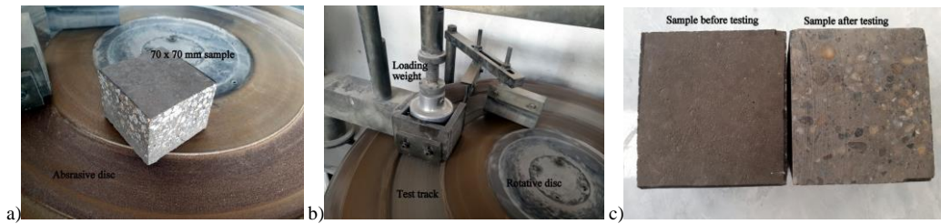
Fig. 4. Böhme abrasion resistance test: a) Sample dimensions; b) Testing of the samples; c) Sample after testing
