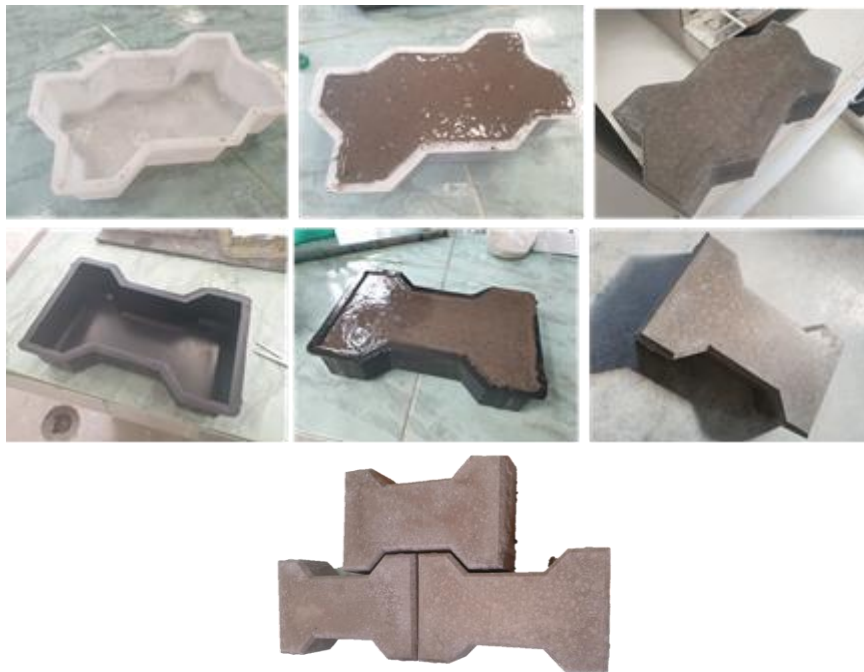
Fig. 3. Production of the alkali-activated fly ash-based geopolymer paving blocks
