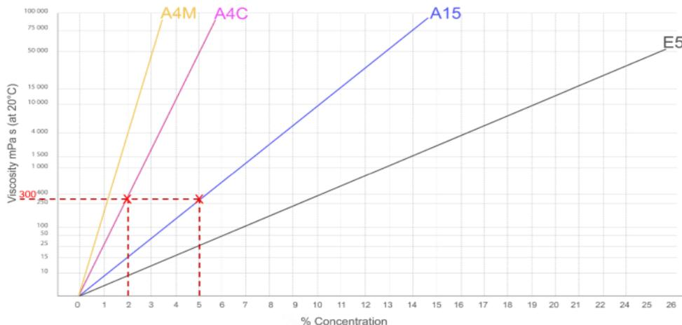
**Fig. 7.** Viscosity graph of methylcellulose.
