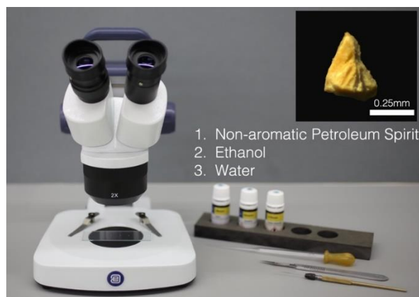
Fig. 4. Stereo microscope with a set of relevant tools and solvents for micro-sampling the substrates that need to be bonded. The tests performed examine the solubility (indirect indication for polarity) and the porosity of the materials in question
