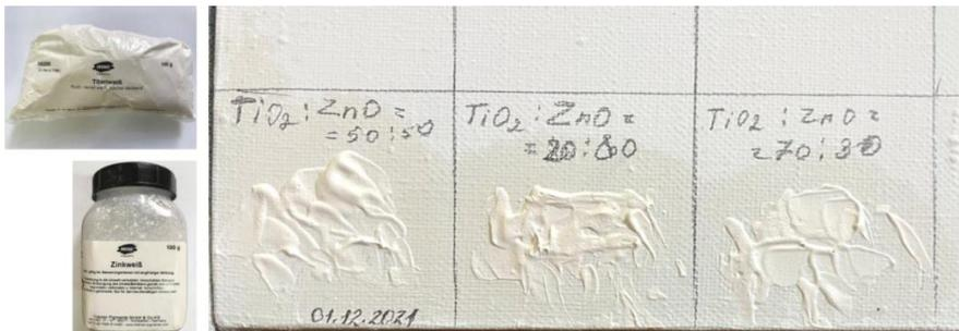
Fig. 2. Titanium-zinc white reference paints out with different TiO<sub>2</sub>/ZnO ratio (in wt.%)
