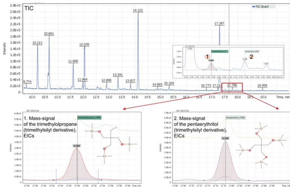
**Fig. 8.** Total ion chromatogram (TIC) of the binder extract of  $\text{TiO}_2$ -based paint from the painting *The Spill on Kerzhenets* by N.M. Romadin. Additionally, the elution areas on the chromatogram of the target components are shown, characterizing the presence of pentaerythritol in the binder composition
