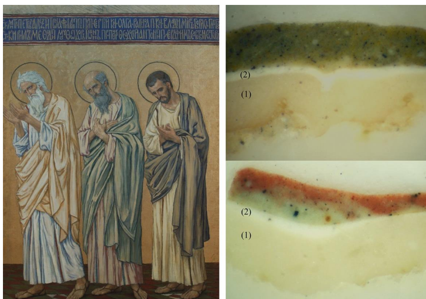
Fig. 8. Cross-sections of the paint layer in the painting The Eucharist by Viktor Vasnetsov. The numbers (1) and (2) indicate the bottom and the upper ground layers, respectively
