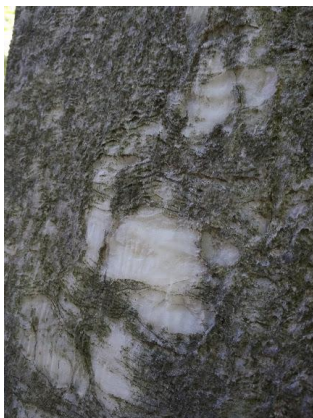
Fig. 3. Dissolution and corrosion of crystalline mass, volume increase of clay component
