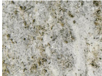
Fig. 22. Micrograph of limewash on the basin of the alabaster baptismal font
