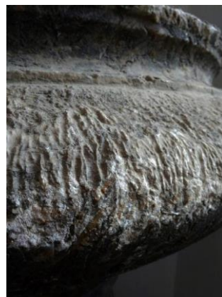
Fig. 11. The flowing water effect. Dissolution of alabaster crystalline mass in the direction of water flow.
