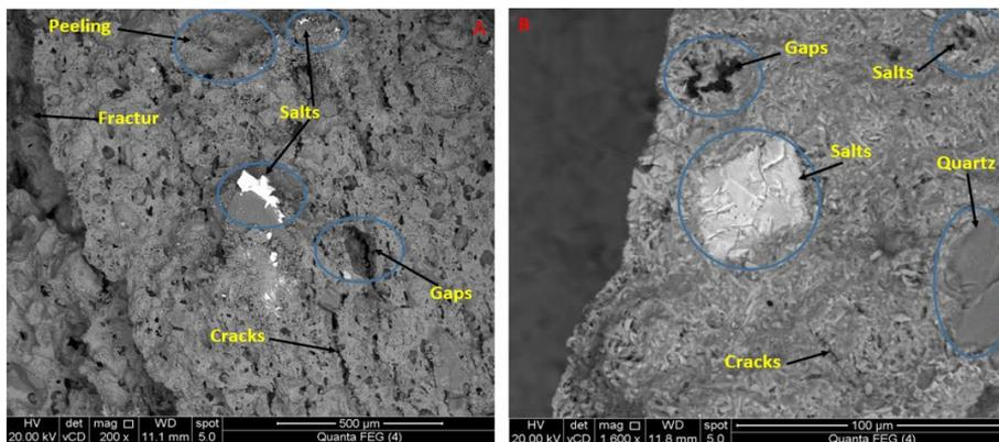
**Fig. 8.** SEM photomicrograph of the first pottery sample:
