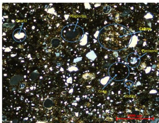
**Fig. 3.** PLM examination of the same pottery sample shows quartz grains, calcite, pyroxene, plagioclase, biotite, grog and iron oxides (10X - CN)
