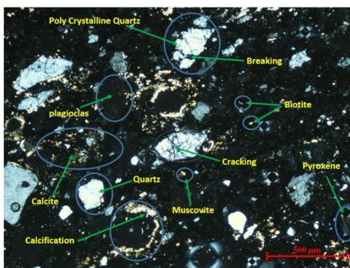
**Fig. 6.** PLM examination of the same sample shows semi-circular and acute-angled quartz grains, polycrystalline quartz grains, limestone powder, plagioclase, some internal cracks, and iron oxide (10X - CN)
