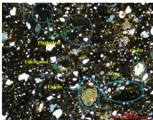
**Fig. 2.** PLM examination of the first pottery sample shows quartz grains calcite, grog, plagioclase, iron oxides, and calcareous deposition (10X - CN)
