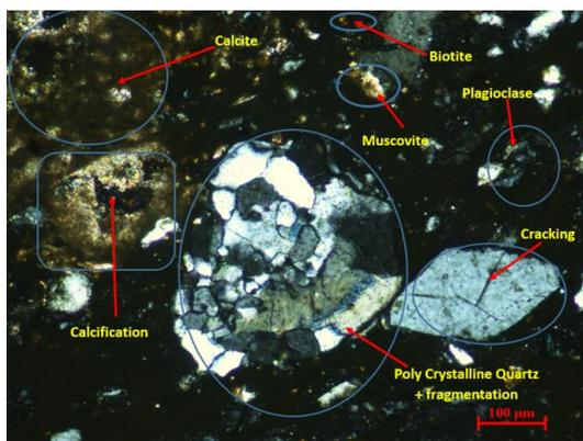
**Fig. 7.** PLM examination of another part pottery sample shows polycrystalline quartz grains, lime stone powder, plagioclase, biotite, muscovite, lime deposit and iron oxide (20X - CN)
