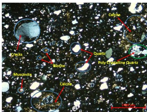
**Fig. 5.** PLM examination of the second pottery sample shows semi-circular and acute-angled quartz grains, calcite, biotite and muscovite, polycrystalline quartz grains and iron oxide (10X - CN)
