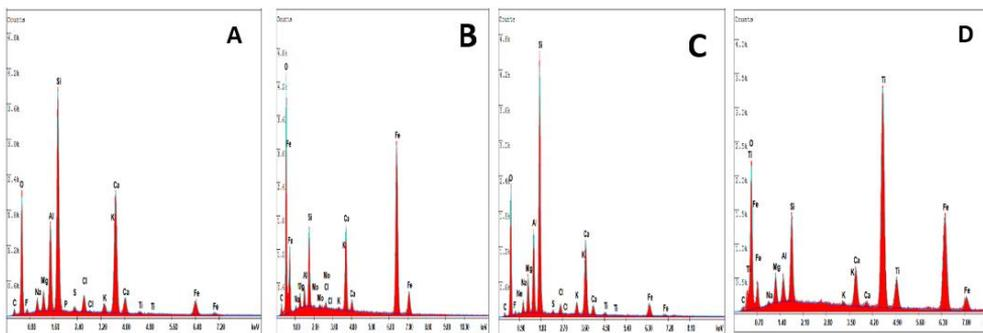
Fig. 10. EDX analysis patterns of pottery samples tell El- Hir, Sinai: A and B - first pottery; C and D - Second pottery
