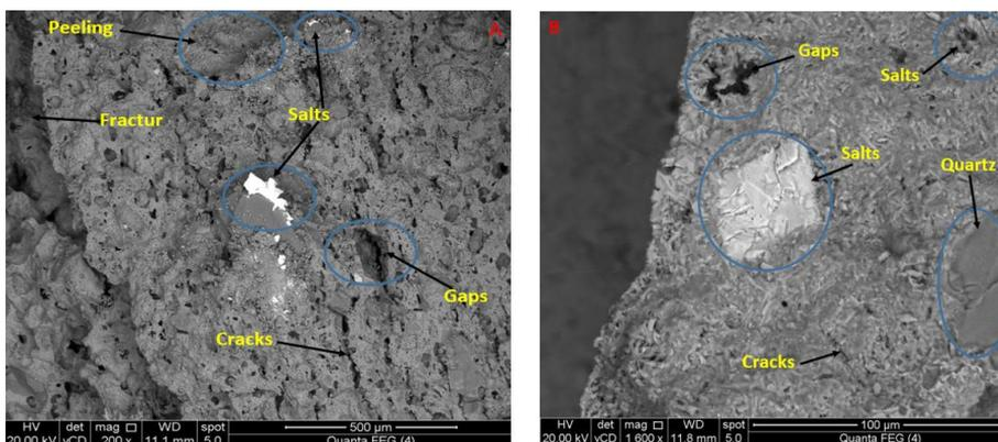
**Fig. 9.** SEM photomicrograph of the second pottery sample:
