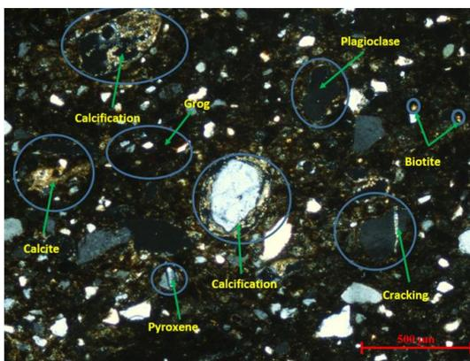
**Fig. 4.** PLM examination of another part pottery sample shows quartz grains, grog, calcite, plagioclase, pyroxene, calcareous deposits and internal cracks in matrix rich in iron oxide (10X - CN)
