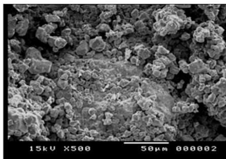
**Fig. 14.** Shows the disintegration of the grains, voids and gaps between the pores of the stone
