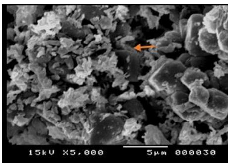
Fig. 25. The formation and flowering of sodium sulfate salts on the membrane of the reinforcing material MTMOS coated for the sample granules
