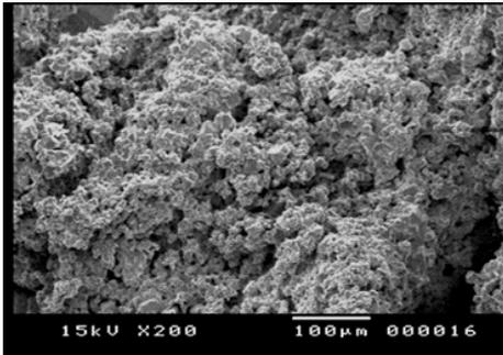
**Fig. 19.** Klucel G is not completely covered with granules
