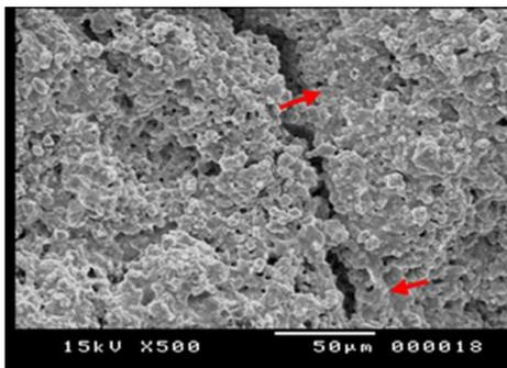
**Fig. 21.** Cracks not filled with Klucel G
