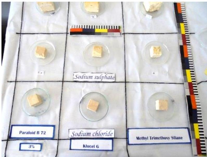
Fig. 5. The reinforced stone samples in the saline solutions
