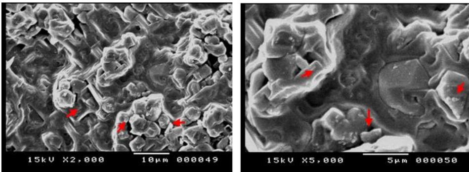
Fig. 29. The formation and flowering of sodium sulfate salts inside the pores and granules of Paraloid B72
