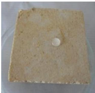
**Fig. 3.** The stone samples absorbing the water drop
