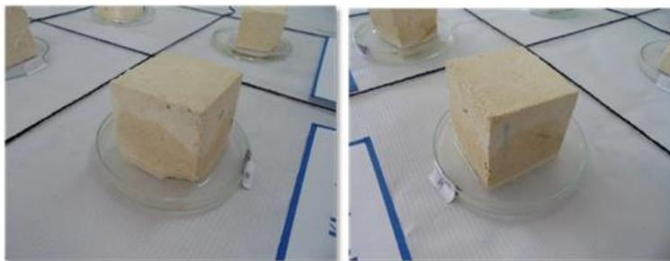
**Fig. 4.** Limestone water absorption
