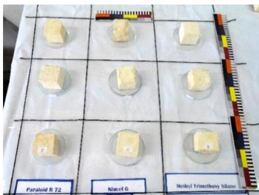
Fig. 1. The preparation of stone samples
