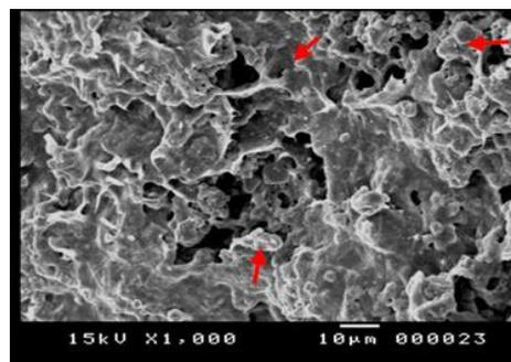
**Fig. 23.** The non-proliferation of Paraloid B72 booster material with blanks and gaps
