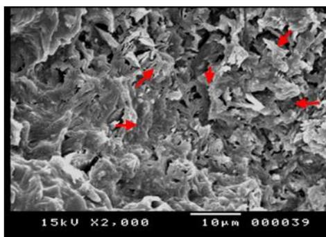
Fig. 27. The formation and flowering of sodium sulfate salts directly above the granules, having the film coated with Klucel G
