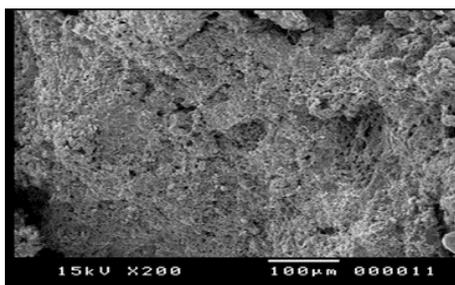
**Fig. 15.** The cracks between the pores of the limestone
