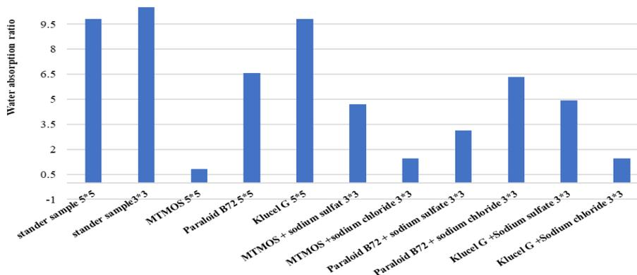
Fig. 11. The results of the water absorption test
