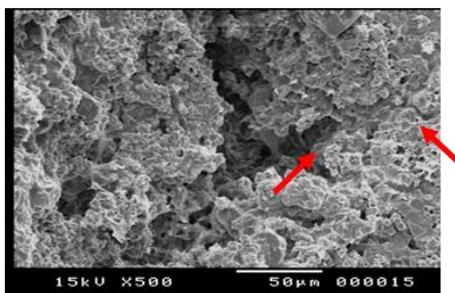
**Fig. 17.** The packing and covering of the granules with the MTMOS consolidation material
