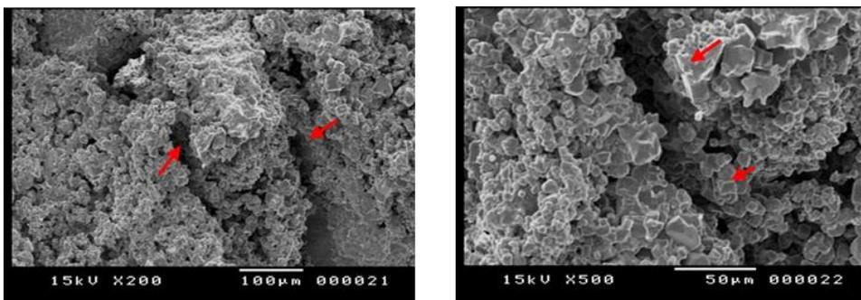
Fig. 24. The cracks are not filled with the Paraloid B72
