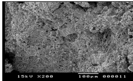
**Fig. 15.** The cracks between the pores of the limestone
