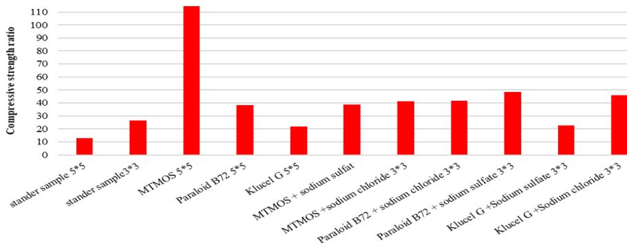
Fig. 13. The results of the pressure test for stone samples after the strengthening process
