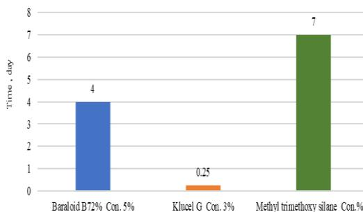
Fig. 10. Showing the time required for water absorption by capillary action
