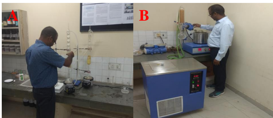
Fig. 1. Preparation of Neem seed extract (A); Evaporation of solvent through rotary vacuum evaporator (B)
