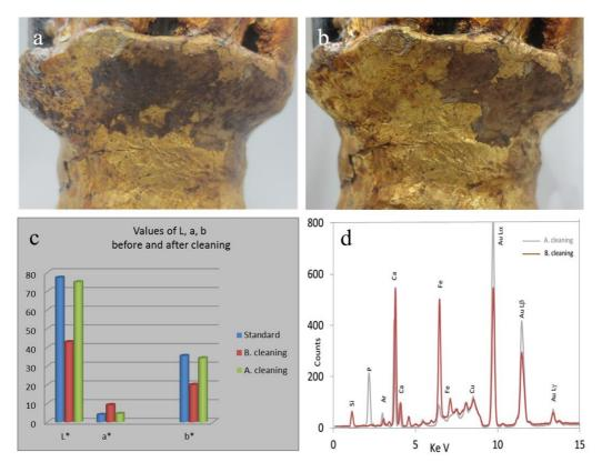
Fig. 7. Gilding surface of drum region of the front left leg with layer of paraffin wax and dirties: a-Before; b- After the gel application; c- Results of colorimetric measurements; d- XRF spectra before and after cleaning
