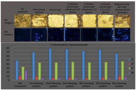
Fig. 5. VIS, UVL imaging and colorimetric measurements for experimental cleaning systems on gilded experimental samples treated with paraffin wax with dirt layers
