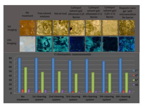
Fig. 1. VIS, UVL imaging and colorimetric measurements for experimental cleaning systems on gilded experimental samples treated with rosin and paraffin wax mixture
