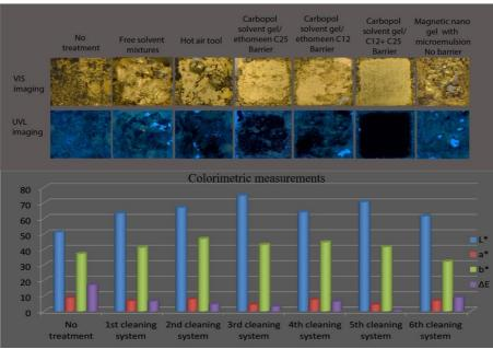
Fig. 3. VIS, UVL imaging and colorimetric measurements for experimental cleaning systems on gilded experimental samples treated with rosin and bees wax mixture with dirt
