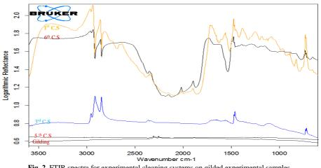
Fig. 2. FTIR spectra for experimental cleaning systems on gilded experimental samples treated with rosin and paraffin wax mixture
