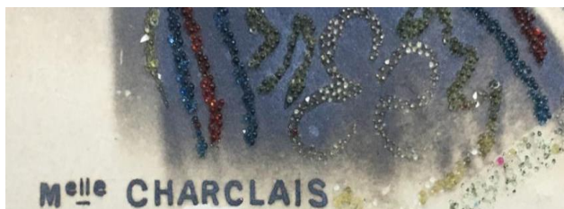
Fig. 3. Silver mirroring caused by the damaging effect of certain chemical reagents on image silver
