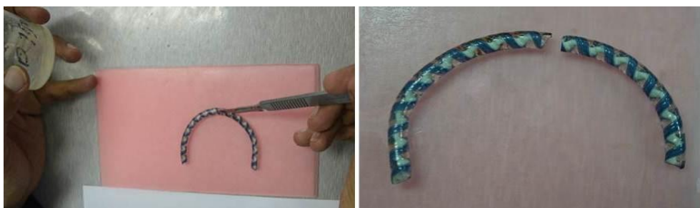
Fig. 10. Glass antique No 2 during adhesive process by Kemapoxy150 3D
