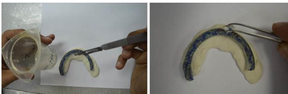
Fig. 9. Glass antique No 1 during adhesive process by Kemapoxy150 3D
