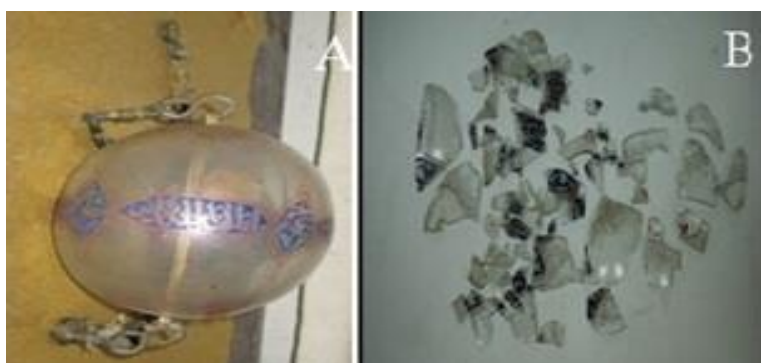
Fig. 4. The case before and after the explosion
