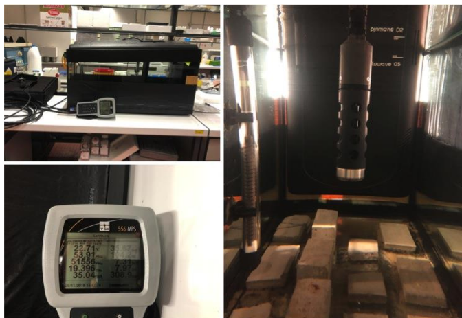
Fig. 3. Arrangement of experimental specimens inside the aquarium and monitoring system of seawater with the multiparametric probe
