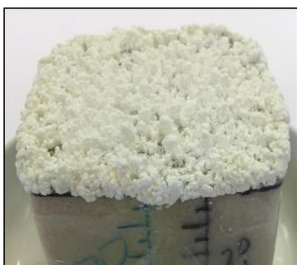
**Fig. 6.** Efflorescences formed at the end of drying process on sample 11-50 salinated with salt mixture and treated with 0.1% inhibitor solution
