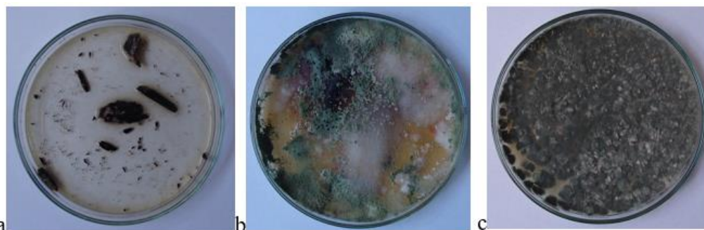
Fig. 4. Fungal growth on wood samples after placement in cultivation media for 8 days of incubation, wood sample prior to incubation (a), after incubation on a MEA medium (b) and after cultivation on a PDA medium (c)
