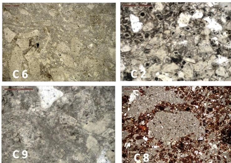
**Fig. 5.** Thin section photomicrographs of the studied stone samples. Scale bar on all images is 200µm and photos taken under plane light except of C8 in crossed polarized light
