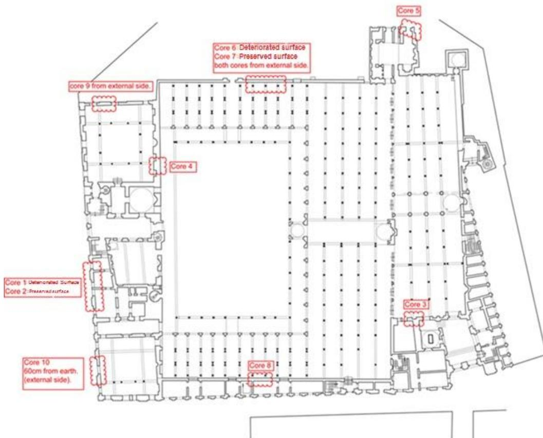
**Fig. 1.** The plan of the sampling location from the different facades of Al-Azhar
