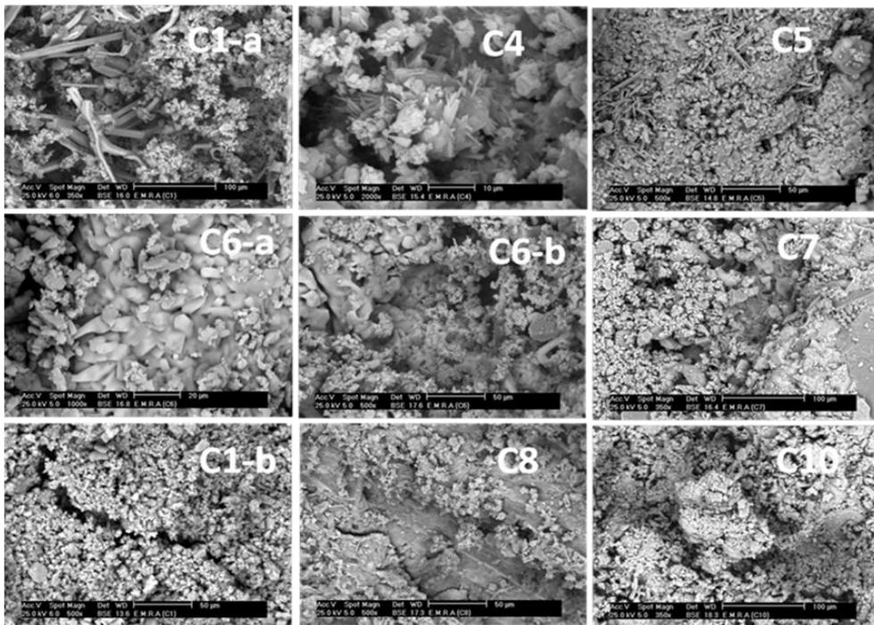
**Fig. 6.** SEM images showed needle shape crystals of gypsum (C1-a, C4 and C5) and halite crystals (C6-a, C6-b and C7). Crystals growing within the stone pores causing micro-crakes (C1-b and C8) and disintegration of the micrite (C10)
