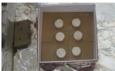
Fig. 3. Samples in the UV lamp compartment
