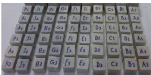
Fig. 8. The specimens with their code number after the consolidation treatment.
