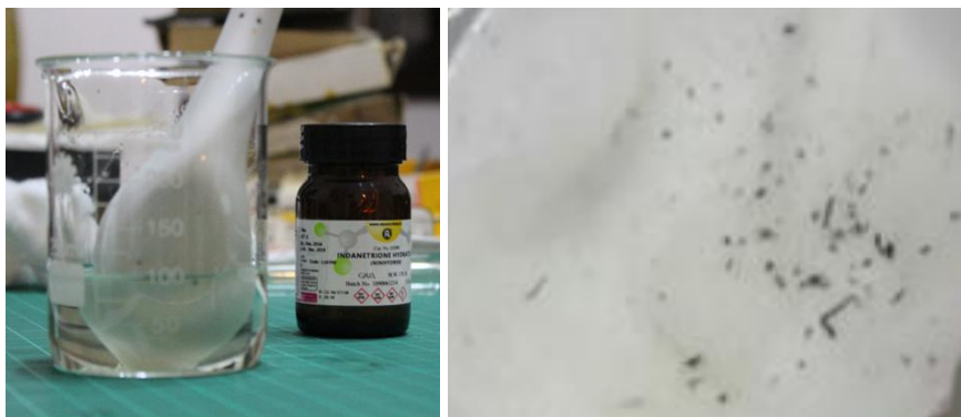
Fig. 11. Ninhydrin test results showed no change for the Faber Castell eraser residues
