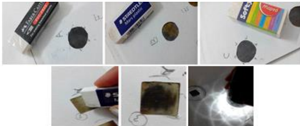
Fig. 4. Erasers tested for mirroring removal/reduction (top). Application method (bottom)
