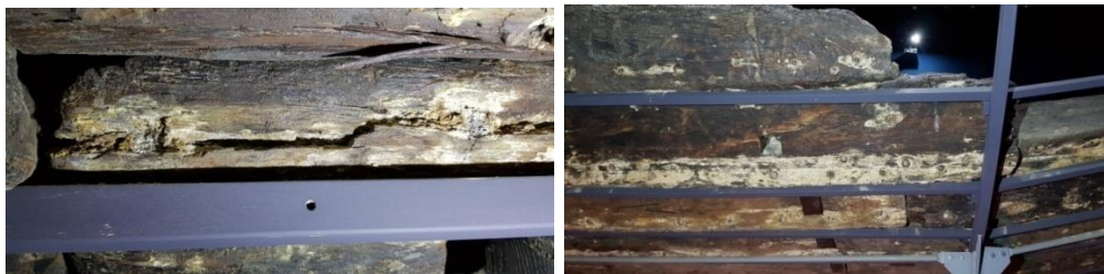
Fig. 2. Acid-degradation symptom observed in the middle part of portside (left) and upper part of starboard (right) of the Shinan wreck. By-products of the acid-degradation crystallized and then destroyed the hull of the wreck
