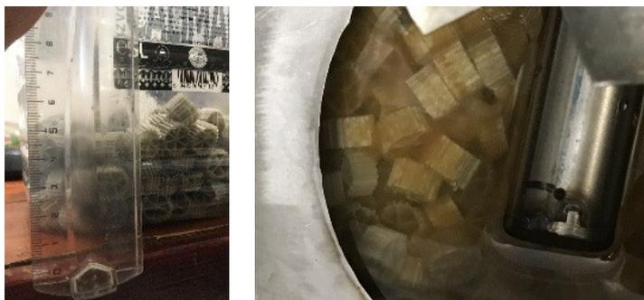
**Fig. 4.** Experimental MBBR stage
