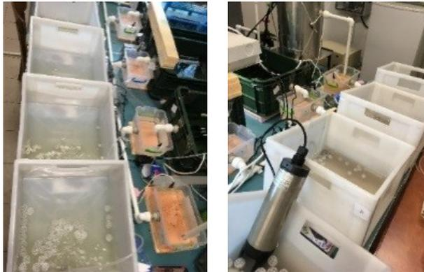
Fig. 7. Experimental tanks to highlight the biofilm attachment on biofilm carriers
