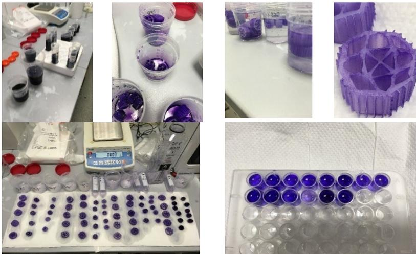
Fig. 8. Experimental tanks to highlight the attachment of biofilm on different biofilm carriers
