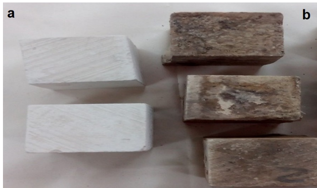
Fig. 5. Illustrates the difference between the cubic samples (a) before and (b) After fungal injection, and weathering.
