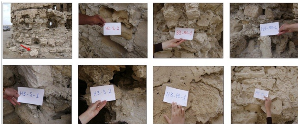
Fig. 3. different sampling processes (stone, mortar and render sampling)
