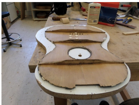
Fig. 5. The top-plate after finishing repair procedure
