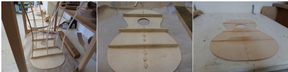
Fig. 15. Bracing struts gluing and forming
