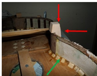
Fig. 7. Ribs – top-plate gluing process
