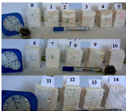
Fig. 6. Photo-documentation for the control R and fourteen limestone samples, treated with the resins under investigation, after 10 cycles of artificial weathering with anhydrous Na 2 SO 4
