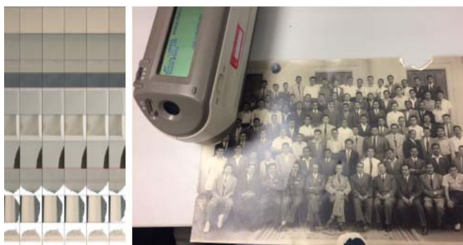
Fig. 4. A printed scale to distinguish the suitable color using a spectrophotometer
