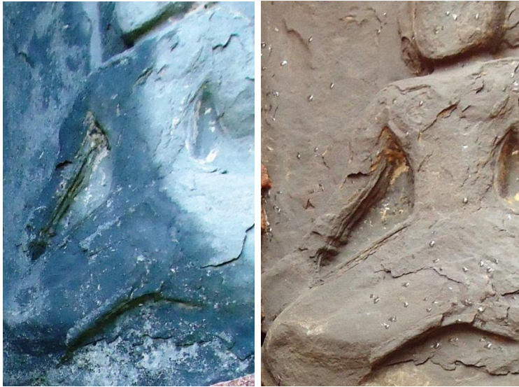
Fig. 5. After preservation of sand stone surface of Sculpture (right) imparting water repellence and un-preserved sandstone surface (left).
