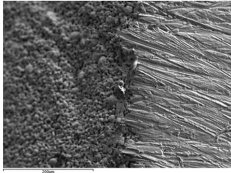
**Fig. 4.** Fired Art Clay™ 650 during polishing
