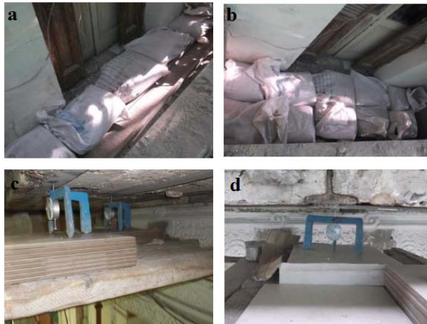
Fig. 18. Static loading test: a. and b. Loading; c. and d. Measuring deflection
