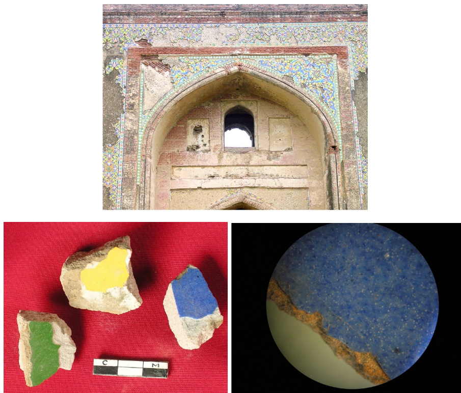
Fig. 2. Close view of decorative art work of glazed tiles, glaze tile samples and photomicrograph image of blue glaze tile
