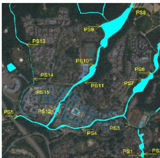
Fig. 7. Location of point source pollution discharge points within IIUM campus
