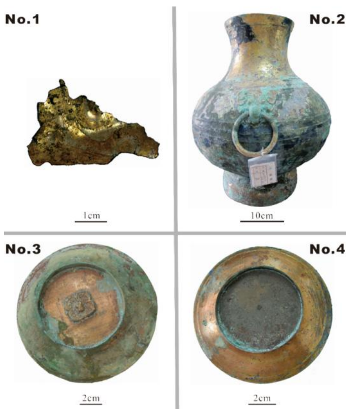
Fig. 7. Samples No.1-4 treated with PCb4 show a shiny metallic luster
