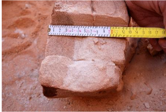
Fig. 11. Area around the Cave of Swimmers. Application of ethyl silicate tested on a sandstone sample.
