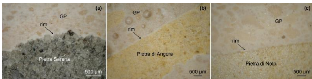
Fig. 1. Stereomicroscope images of samples prepared with natural ornamental stones: a) Pietra Serena; b) Pietra di Angera; c) Pietra di Noto. The rims are indicated by arrows.
