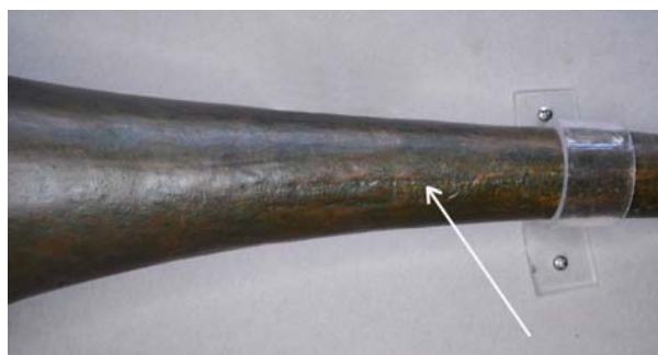
Fig. 4. Detail of the bell in cornu 286788. The arrow indicates the braze welding presumably made by brass.
