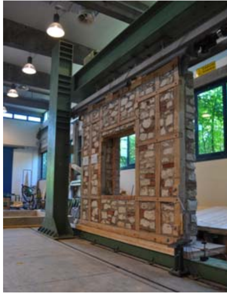
Fig. 7. The full scale sample of Borbone constructive system tested under quasi static cyclic loading
