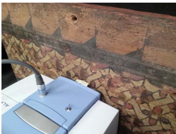
Fig 2. Instrumental setting for the Total Reflectance IR measurements.
