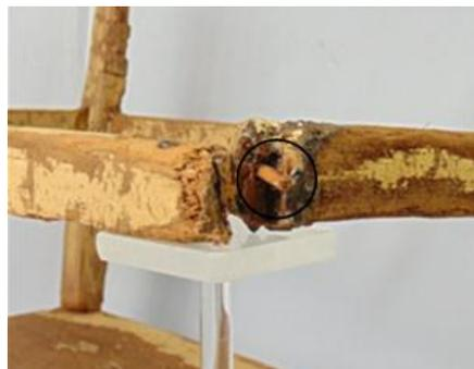
**Fig. 4.** A previous new dowel used in assembly of offering table.
