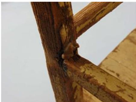
**Fig. 3.** A thick bulk of previous preservation and restoration material, at the connecting point between the front rail and front
