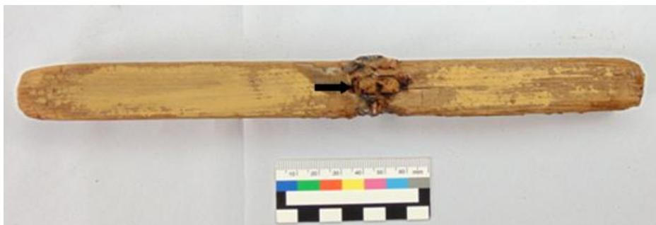
**Fig. 7.** Left front leg separated from the offering table and remains of broken tongue in mortise as shown by arrow.
