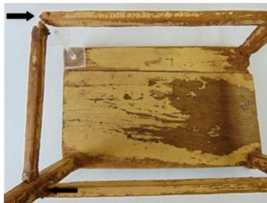
**Fig. 6.** Broken tongues in front and back rails.
