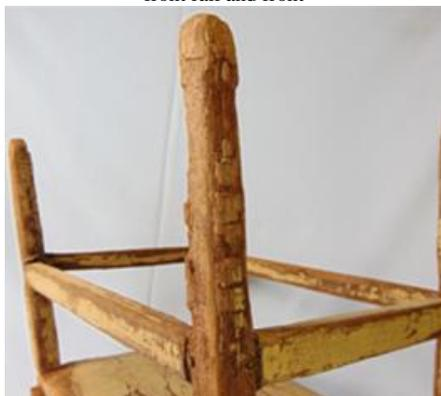
**Fig. 5.** Horizontal cracks and cubic breaks due to Fungal
