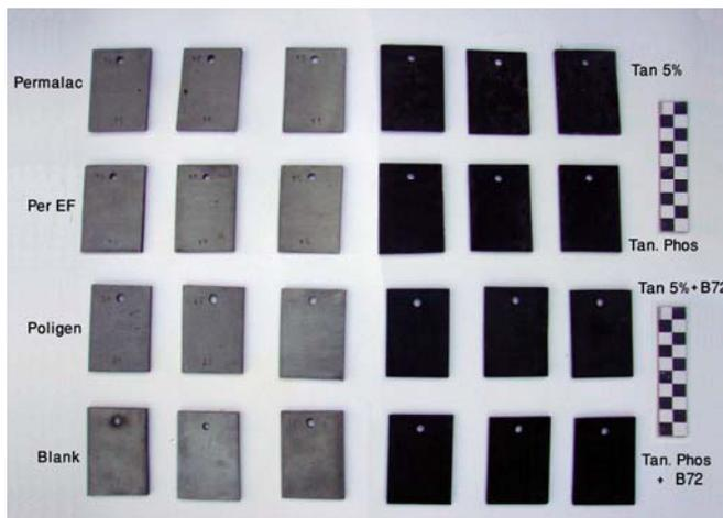
**Fig. 2.** The cast iron coupons after applied the protection systems.
