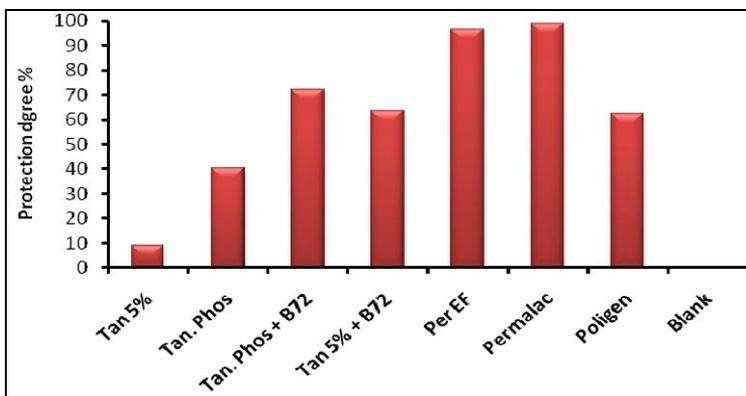
**Fig.8.** The protection degree (%) of the selected protection systems after eight months of exposure.
