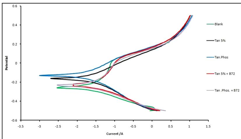
Fig. 5. Polarization curves of cast iron samples treated with different inhibitors compared with untreated sample.
