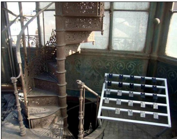
**Fig. 3.** The rack with the whole cast iron coupons were exposed inside the clock tower of Muhammed Ali's mosque in Salah El-Din Citadel in Cairo.
