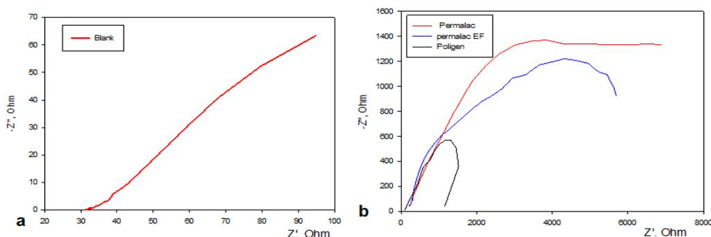
**Fig. 6.** Electrochemical impedance spectroscopy (EIS) of: **a)** uncoated cast iron, **b)** cast iron coated with Permalac, Permalac EF and poligen at open circuit potential at 25 °C.
