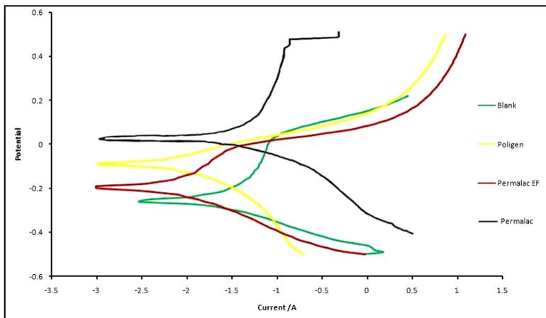
Fig. 4. Polarization curves of cast iron samples treated with different coatings compared with untreated sample.
