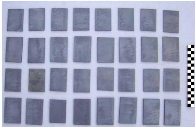
**Fig.1.** The cast iron coupons after the final preparation.
