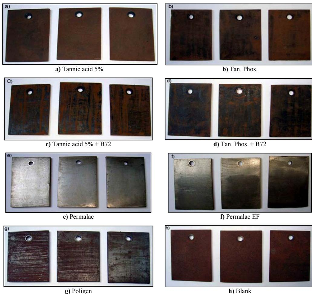
Fig. 7(a- h). Macrographs show assessment of the behavior of the protection systems after eight months of exposure.
