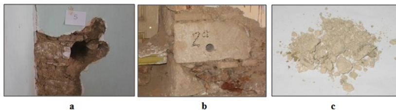
Fig. 12. Precise locations of sampling specimens D7-MS (a) and D10-LS (b), and physical state of mortar sample (c).
