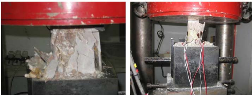
Fig. 16. Testing of the samples: cube and cylinder
