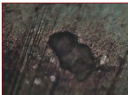
Fig. 5. Micrograph of a sample from the coin no.7 shows a block of lead in the alloy and the elongation of grains (150X).
